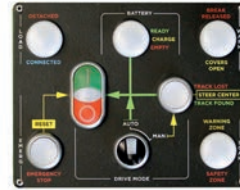
Controle console with buttons Manual/automatic, start, stop, reset, steering central Item number OPT0177
